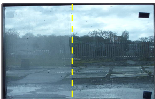
Glass after exposure to dust Right side is treated and is dust free
